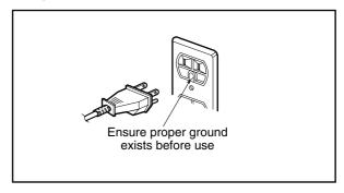
For a permanently connected appliance: This appliance must be connected to a grounded, metallic, permanent wiring system, or an equipment grounding conductor should be run with the circuit conductors and connected to the equipment grounding
